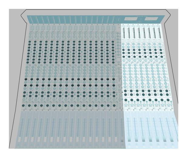
The Group section of the console greatly enhances the flexibility of the TRIDENT 88 console and provides a number of different functions. There are 8 Group modules provided on the console, each controlling the associated group mix bus outputs. The groups can be used as audio subgroups for combining and processing a collection of input channels. Each group bus has its own TRS Insert jack and TRS balanced Output jack on the rear Master Connector panel.
