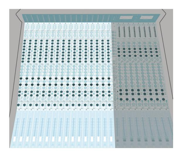
The TRIDENT 88 Input module is an extremely sophisticated and flexible channel that can be used for recording, mixing and monitoring multi-track recordings. It will accept a signal from a low impedance balanced microphone, high or low level balanced line input, or even the output from a musical instrument.
