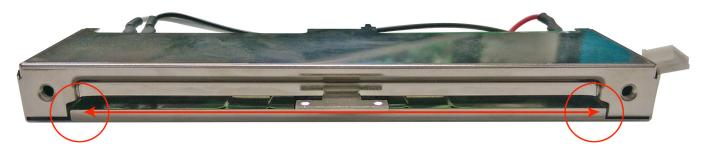
**Figure 1:** Start by blowing one end, and then the other. There is usually dust or debris in the fader that will come out easily, and this usually would be all that is needed in terms of cleaning. Move the fader carriage to one end and blow air into the slot aiming away from the carriage so that dust can escape through the slot. Then move the carriage to the opposite end and blow air aiming the opposite way.
